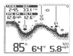
The time, speed, and distance calculations are useful for tracking your progress on a trip. The input voltage is useful for determining the condition of the charging system of the boat.
